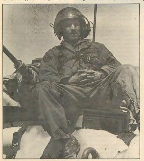
M60 tanker relaxes against M85 .50-caliber machine gun. He is sitting on the gunner's periscope.
